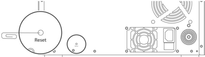
To revert to the default password, use a pin to press the Reset button for three seconds or until you hear a short beep – – en
